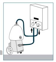
If the pump is not used for a long time, it will be blockaged. To avoid this, run the pump once a week.
